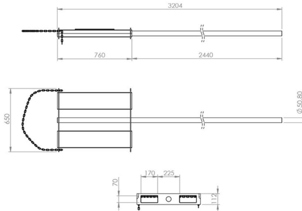
**19263 EIXO P. TRANSPORTE DE BOBINAS P. EMPILHADEIRA**
